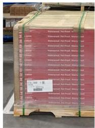
Unit load doesn't use any metal packaging components
